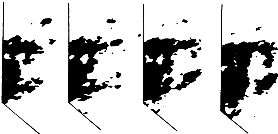
FIGURE 1. Four successive slices of a computer-generated approximation to the volume B(P) > 0 , where B(P) is the Gaussian approximation to a Burgers scalar field at a point P in space. Clearly, these drawings are much too smooth to represent actual turbulence (see figure 2), but it has not escaped the author's attention that they are reminiscent of various portions of the earth's surface: Greece, the Sea of Okhotsk (as seen in a mirror), the Gulf of Siam or perhaps Western Scotland. In other publications, the author has shown that, while such a resemblance is in no way unusual, many other parts of the world are smoother, and require a fractional Brownian model with a larger value of H than either of the two which occur in turbulence. Note that, although the black and white regions are identical in their statistical properties, the white one is by far the larger. The above graphs do not include such 'empty' portions of the square slices.
